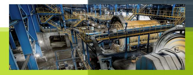
The monitoring system is installed on the ball mill with a monitoring unit including temperature, vibration, sound, load and other parameters.
